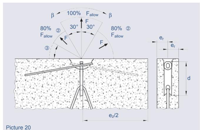
The diagonal tension reinforcement has to be positioned close to the recess former.
