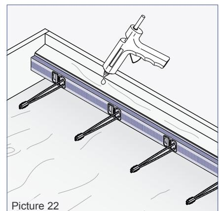
For elements with the same height, it is recommended to start the installation at the upper element edge. This allows a concreting of the rail-free part at the lower element edge. Alternatively, for the rail-free part a simple timber board can be installed to get a continuous grouting channel.
