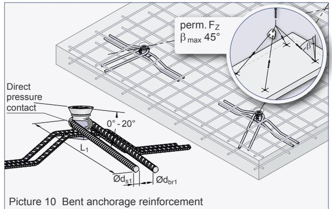
Picture 10 Bent anchorage reinforcement
