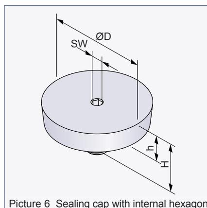
Picture 6 Sealing cap with internal hexagon
