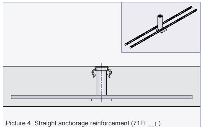
Picture 4 Straight anchorage reinforcement (71FL\_\_L)
