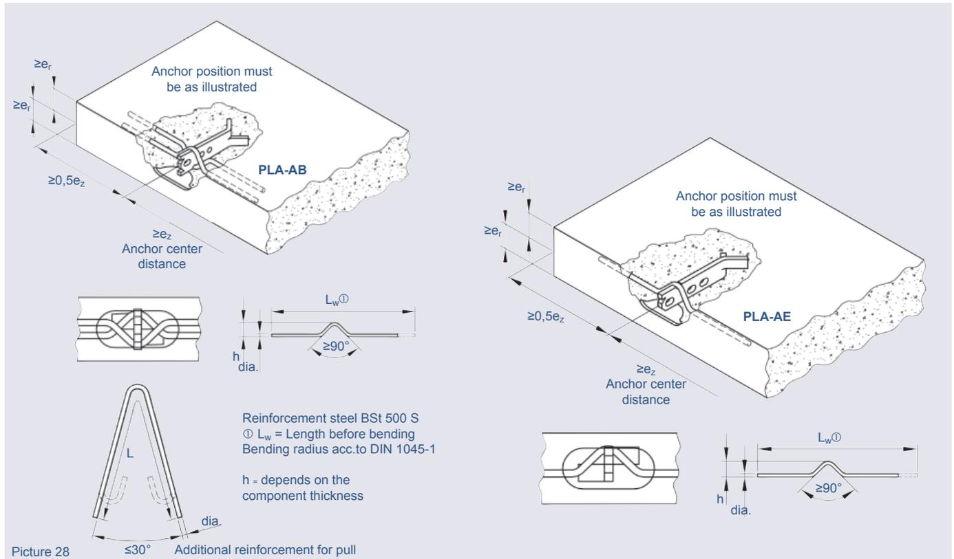
The horizontal legs of the tilting and turning reinforcement are located directly within the outermost position of the reinforced area. Tilting reinforcement on both sides also acts as angled pull reinforcement. No additional angled pull reinforcement is required.
