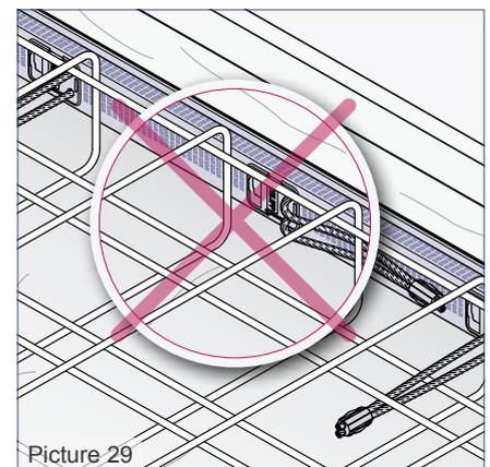
The function of a lapped splice can only work if a maximum vertical distance of 20 mm between the loops is not exceeded.
