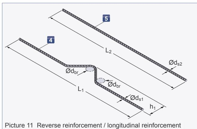
Picture 11 Reverse reinforcement / longitudinal reinforcement
