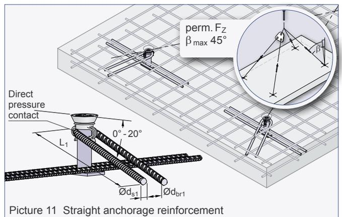
Picture 11 Straight anchorage reinforcement
