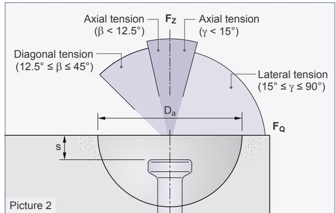
The Spherical head anchor is part of the PHILIPP Transport anchor system and complies with the VDI/BV-BS Guideline "Lifting inserts and lifting insert systems for precast concrete elements" (VDI/BV-BS 6205).
