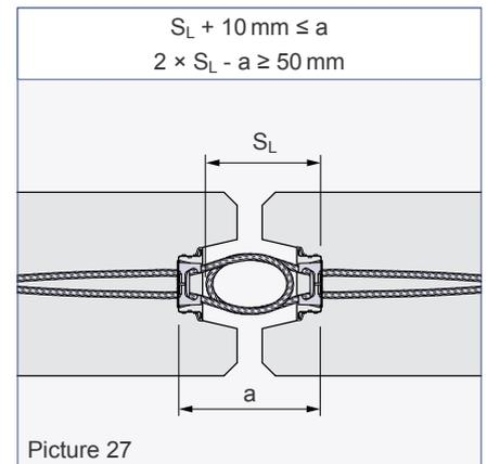
In thin concrete units it is possible to bend the end of the loop under consideration of the bending radius. To simplify the bending of the wire rope a rebar  $\text{Ø}8$  mm shall be installed.
