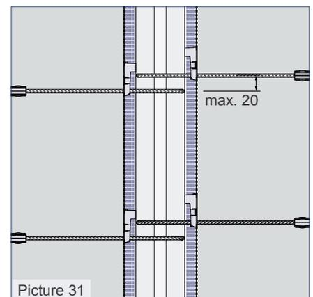
The plastic cover of the installed rail must be released at one rail end. Then, it can be removed easily from the rail. The loops are now folded right-angled to the (metal) box or rail.
