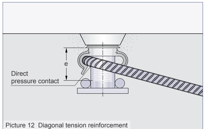
Picture 12 Diagonal tension reinforcement
