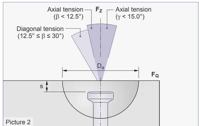
A Spherical head anchor with offset balances an inclination of reinforced concrete sandwich panels during lifting and mounting.
