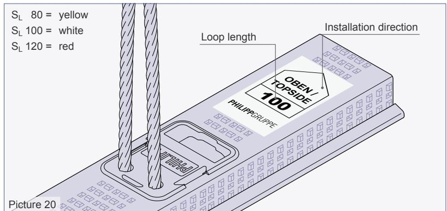
The Connecting rail can be fixed by nailing or hot bonding to the formwork.
