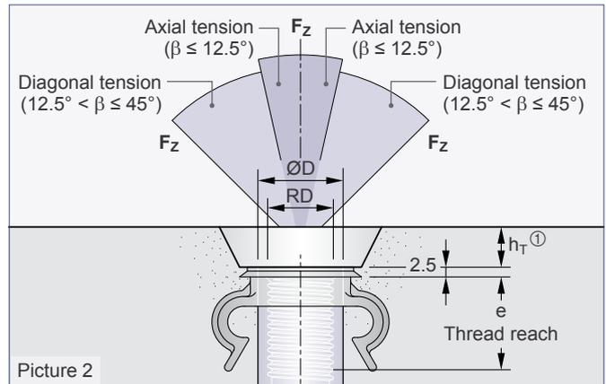
The Capped end anchor is used for installation in slab-like elements. It is part of the PHILIPP Transport anchor system and complies with the VDI/BV-BS Guideline "Lifting inserts and lifting insert systems for precast concrete elements" (VDI/BV-BS 6205).
