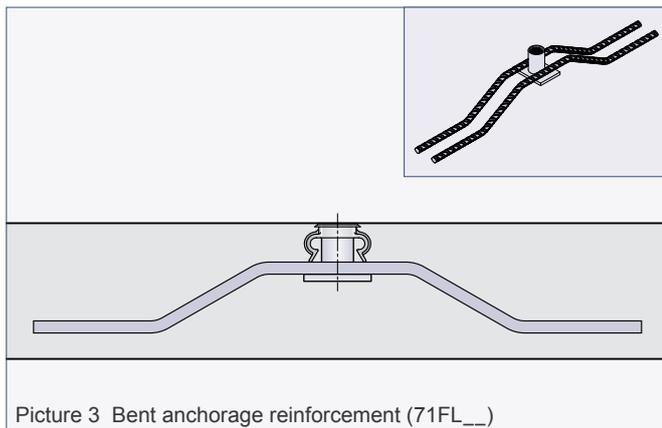
Picture 3 Bent anchorage reinforcement (71FL\_\_)
