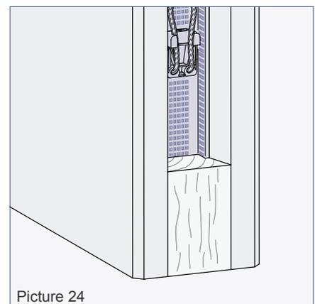
Like the Connecting loops also the Connecting rails can be produced as a special version for lightweight concrete (e.g. 84VS201005LB). In this case, to the reference number „LB” must be added.
