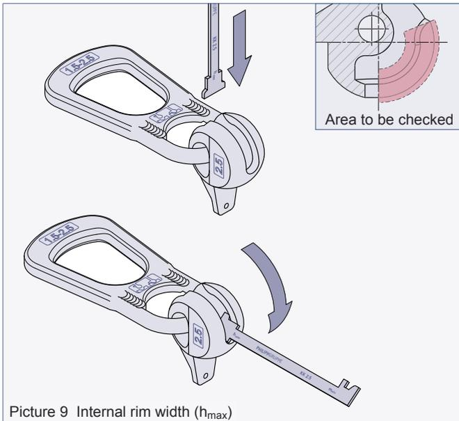
Picture 9 Internal rim width ( $h_{max}$ )
